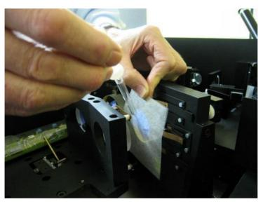
Apply clean alcohol or acetone via a fine pipette to a lens tissue held as low as possible and touching the mirror. The fluid should wet the tissue so that it adheres to the whole mirror area. No excess fluid should be allowed to drip down.
