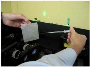
In a normal environment the interferometer mirrors do not need to be cleaned very frequently. After a period of 2 or 3 years the front surface of the mirrors may however begin to show excessive scatter loss.
