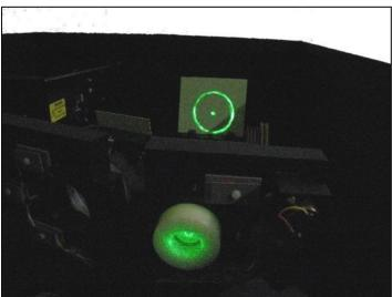
FP1 is now set at the correct calibration distance. This distance depends on the laser wavelength used and can be found in section 3.6.2 of the manual. Adjust the dial gauge to read this value.
