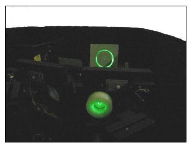
Set the Z-control so that the disc is at maximum intensity, and then change Z until the ring is maximum. Note the direction that you turned the Z-control to go from disc to ring. If the direction was clock-wise the spacing of FP1 is slightly too large. Adjust the mirror spacing by tapping the switch on the motor control – each tap will change the spacing by 0.5µm or so. Continue until the disc and the ring reach maximum brightness for the same setting of the Z-control.
